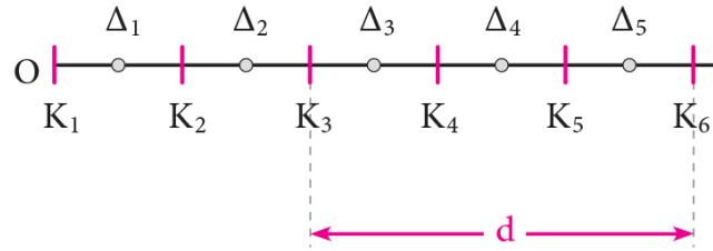
$$d = \frac{\lambda}{4} + \frac{\lambda}{2} + \frac{\lambda}{2} \Rightarrow d = \frac{5\lambda}{4} \Rightarrow 4d = 5 \frac{v}{f} \Rightarrow f = \frac{5v}{4d} \Rightarrow f = 5Hz.$$
