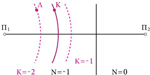
$$\text{Είναι } r_{1K} - r_{2K} = -10\text{cm} = -1\lambda \Rightarrow \lambda = 10\text{cm}.$$
