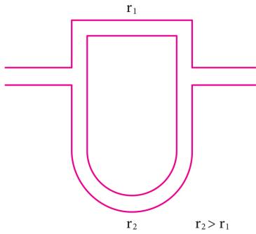
$$r_2 - r_1 = \pi R - (2R + 2x) = N\lambda > 0 \Rightarrow (\pi - 2)R + 2x = N\lambda \Rightarrow$$
