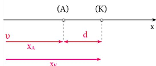
$$\begin{cases} f1: \Delta\varphi_1 = 2\pi \frac{\Delta x}{\lambda_1} \Rightarrow \Delta\varphi_1 = 2\pi \frac{d}{v} \cdot f_1 \quad (1) \\ f2: \Delta\varphi_2 = 2\pi \frac{\Delta x}{\lambda_2} \Rightarrow \Delta\varphi_2 + 2\pi = 2\pi \frac{d}{v} \cdot f_2 \quad (2) \end{cases}$$
