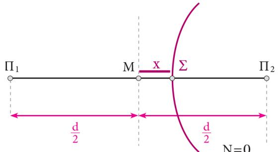
$$\text{Για το } \Sigma: r_1 = \frac{d}{2} + x, r_2 = \frac{d}{2} - x \Rightarrow r_1 - r_2 = (2N + 1) \cdot \frac{\lambda}{2}, \mu\epsilon N = 0$$
