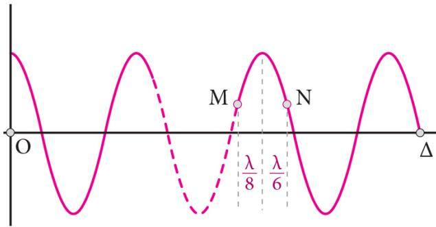
$$A'_M = \left| 2A \cdot \sigma v v 2\pi \frac{x_M}{\lambda} \right| = \left| 2A \cdot \sigma v v 2\pi \frac{\kappa \frac{\lambda}{2} - \frac{\lambda}{8}}{\lambda} \right| = 2A \left| \sigma v v 2\pi \left( \frac{4\kappa - 1}{8} \right) \right|$$
