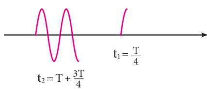
$$\Delta t = t_2 - t_1 \Rightarrow \Delta t = \frac{3T}{2}, \Delta \varphi = 3\pi = 2\pi \frac{\Delta x}{\lambda} \Rightarrow 3 = 2 \frac{12}{v \cdot T} \Rightarrow$$
